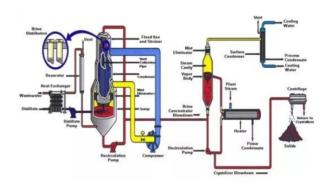
The basic structure of a properly functioning ZLD system comprises of the following components:
